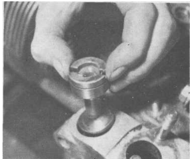
6.8a Replacing the distributor drive shaft. Note the fuel pump drive cam on the shaft
