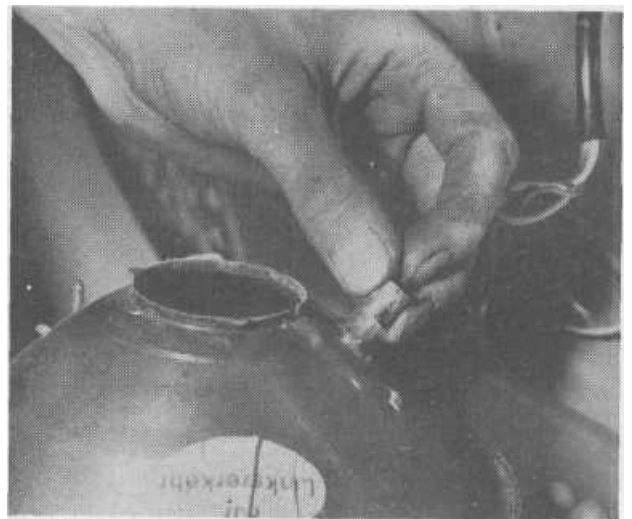
25.2 On some models the parking lamp is in the head light reflector
